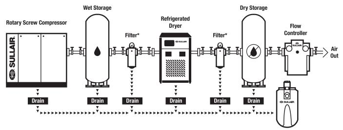
\* Models RFE-03 through RFE-459 include integrated filters. Models RFE-555 through RFE-2083 require a pre- and after-filter as shown.
